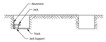
Pits are excavated on each side. The jacks will bear against the back of the left pit so a steel or wood abutment is added for reinforcement. A simple track is added to guide the concrete pipe sections. The jacks are positioned in place on supports.
