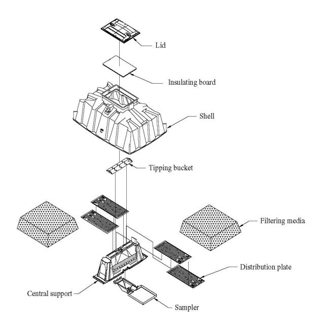
Exploded view of the system ST fiberglass models
