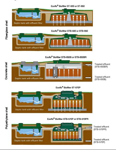
The **Ecoflo® Biofilter's** operating principle allows the system to be used continuously or intermittently without requiring any particular precaution and without impacting the performance of the system. No action is required from the owner to start the system.
