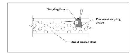
Take care not to touch the lip of the sampling tray with the sampling device when installation and removal.
