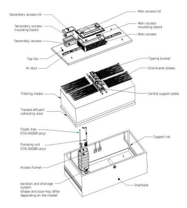
Exploded view of the system Concrete models
