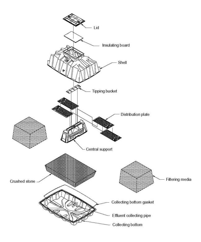
Exploded view of the system STB fiberglass models
