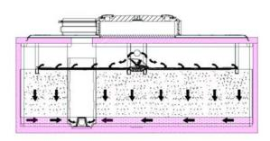
Water flow diagram (STB-650B discharge by gravity)
